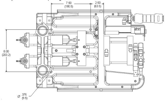
Figure 1: Mounting Hole Dimensions for Installing the PR70 Machine (dimensions in inches/mm)
